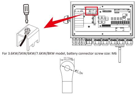
DC Battery Input 1/2AWG Wire Size
