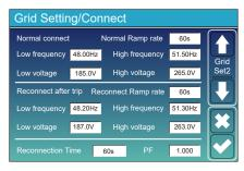
Normal connect: The allowed grid voltage/frequency range when the inverter first time connect to the grid.
