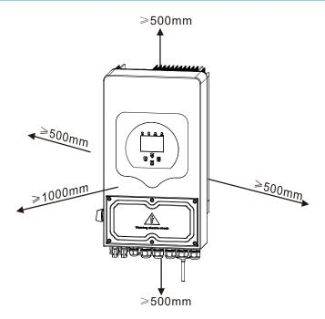
For proper air circulation to dissipate heat, allow a clearance of approx. 50cm to the side and approx. 50cm above and below the unit. And 100cm to the front.
