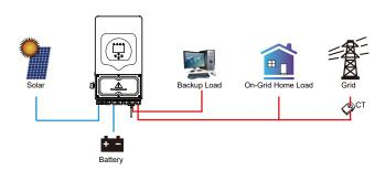
**Solar Sell:** "Solar sell" is for Zero export to load or Zero export to CT: when this item is active, the surplus energy can be sold back to grid. When it is active, PV Power source priority usage is as follows: load consumption and charge battery and feed into grid.
