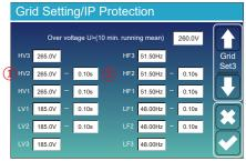
HV1: Level 1 overvoltage protection point;
