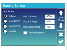
**Battery capacity:** it tells Deye hybrid inverter to know your battery bank size.
