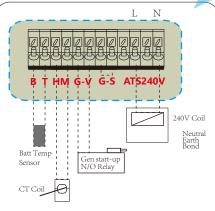
BT: battery temperature sensor for lead acid battery.
