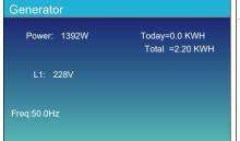
This page tells generator output voltage, frequency, power. And, how much energy is used from generator.
