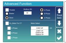
**Ex\_Meter For CT:** when in Three phase system with CHNT Three phase energy meter (DTSU666), click corresponding phase where hybrid inverter is connected. e.g. when the hybrid inverter output connects to A phase, please click A Phase.
