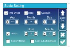
Factory Reset: Reset all parameters of the inverter. Lock out all changes: Enable this menu for setting parameters that require locking and cannot be set up. Before performing a successful factory reset and locking the systems, to keep all changes you need to type in a password to enable the setting.
